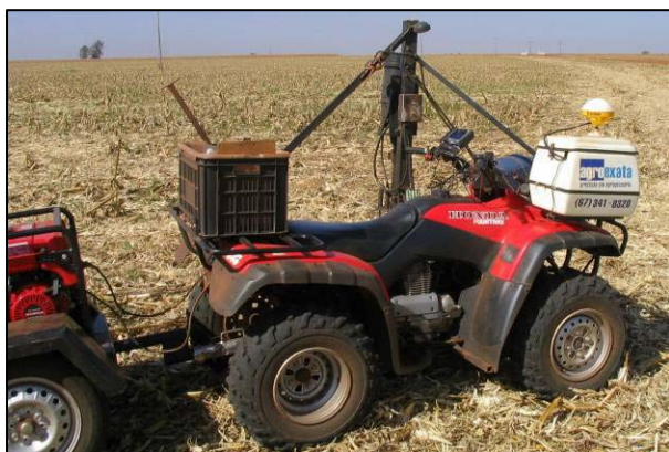
ATM-mounted automated soil sampling equipment used by AgroExata.
